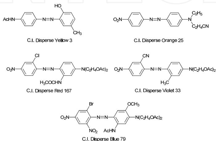
Fig. 5. Some typical azo disperse dye structures.
